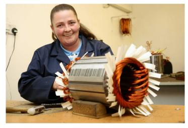
varnish. Each winding is then subjected to 2000V-to-earth flash test, ohms readings are taken with a multi-meter and recorded, and then the winding is subjected to a full load test on a transformer.
