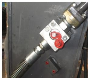
Hydraulic hose is now connected to B-Quick coupler.
