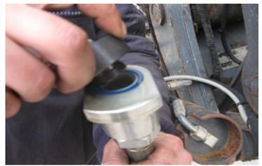
Protection plugs for hydraulic hoses have special for the oil from hose. When closing a hose with our plug, there is no oil spilling because all oil goes to this container.
