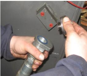
Remove protection plug from the Hammer's hydraulic hose
