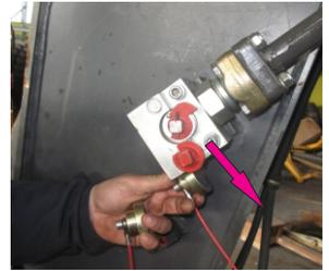
Remove protection plug from the B-Quick coupler
