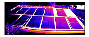
Untouched infrared photos show water (blue) inside a fully filled competitive system. Uneven flow leaves hot spots (red) that reduce heating performance.
