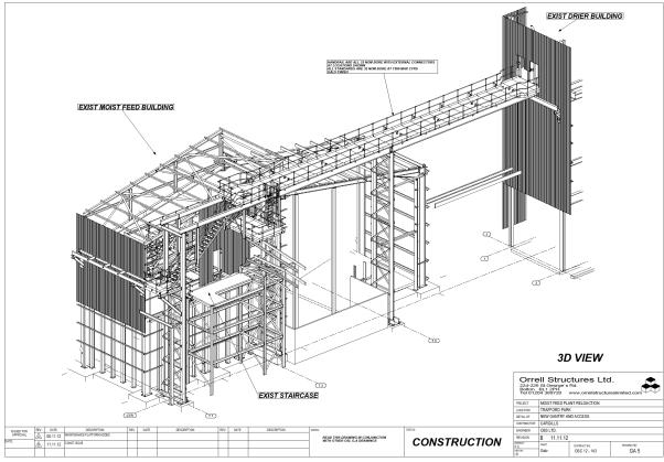
Structural steelwork and metal work, project value £100K steel weight 30T, new conveyor support steelwork and internal platform.
