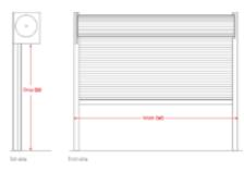
PLEASE NOTE: There must be a suitable surface for the headrails to attach to - e.g. a joist, lintel or beam. If one of these is not in place, one must be fitted. If in doubt, please contact us.
