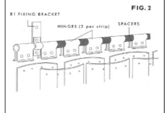
Each PVC strip should be trimmed 20mm above floor level to allow it to hang freely.
