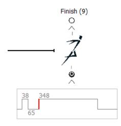
TSS is an **intelligent system**. TSS is able to recognise the interruptions of the beam caused by different body parts while **evaluating only the interruption caused by the torso** of the athlete, making it one of the most accurate systems on the market.
