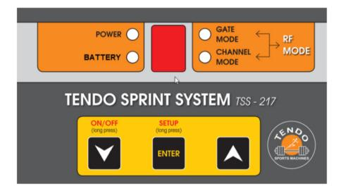
Immediately after the ON/OFF button is released, information about a current setting of the photocell is shown on a LED display for 5 seconds.
