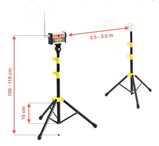
reflector pairs in height of 100 - 110 cm from the ground). Make sure that the photocells and reflectors are in the same height so the beam of the photocell falls in the middle of the reflector.
