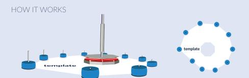
Define the space of the FLOWER by using ground template. Install retractable central pole and perimeter stands. Perimeter stands can be fixed to the ground, or weighted by using water ballast bags (weight from 170kg per stand). There are triangle water ballast bags included in a base platform of central pole too.
