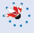
Pre-inflate all petals, zip on the artwork (in case of banner version) and hang on petals one by one to the central pole. Starting with the biggest one, retract central pole by installation of other petals one by one. Inflate each petal to the full pressure after its installation.
