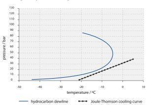
Each certificate of calibration for hydrocarbon mixtures includes a phase diagram calculated using equations of state showing how the stated storage and usage temperature have been derived.
