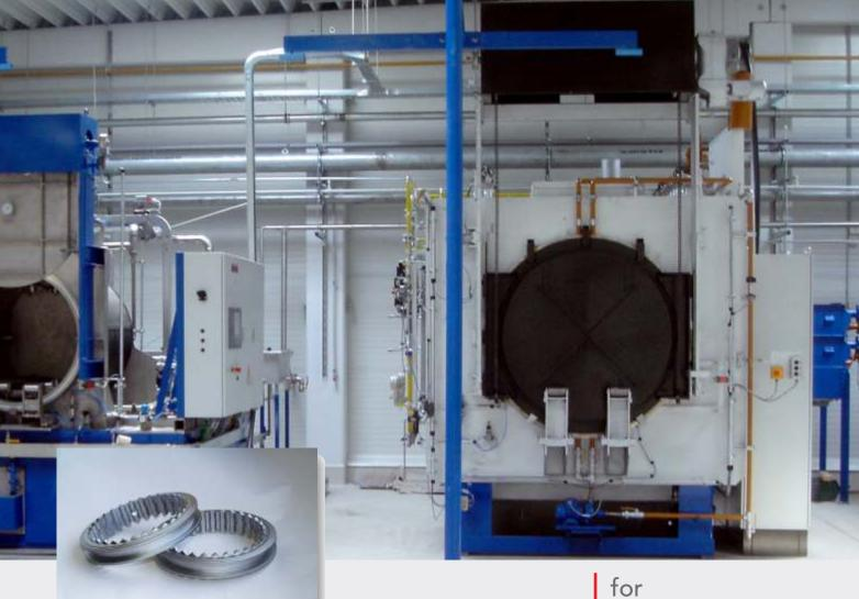
for gas-nitriding nitrocarburizing with nitriding potential control system steam oxidation bright annealing
