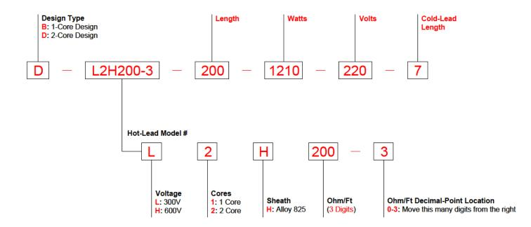
The model shown above is: Design D, Rated 300V, 2-Core, Alloy 825, 0.2 Ohm/ft, 200', 1210W, 220V, 7' Cold-lead.
