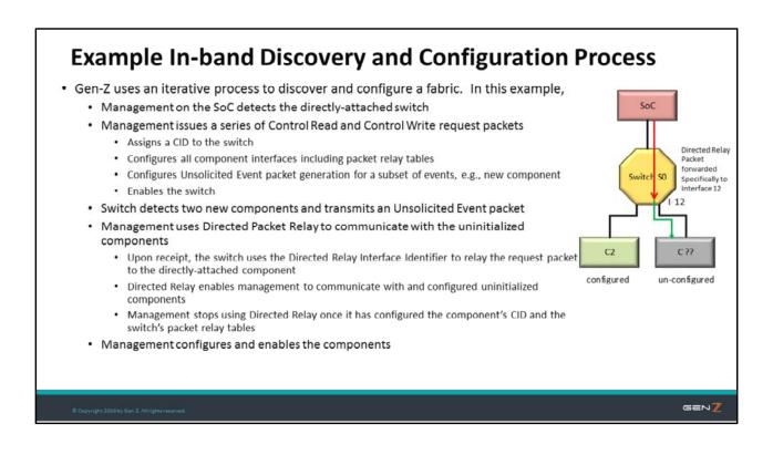
To communicate with uninitialized components within a switch topology, management sets the Directed Relay Interface Identifier field in Control Read and Control Write request packets to inform the switch which egress interface to relay the packet through to the component. This enables the switch to proxy request and response packets on behalf of the uninitialized component.
