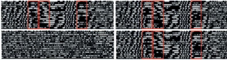
Figure 21.7: Spectral fingerprints of different materials. Channels are oriented vertically while frequency increases from left to right. Top right: No specimen. Bottom right: Aluminium sheet, resulting in noise. Top left: 1 mm ABS sheet. Bottom left: 1 mm PP sheet. Areas containing distinguishing features are highlighted. Signals are intentionally overdriven to enhance visibility of features.
