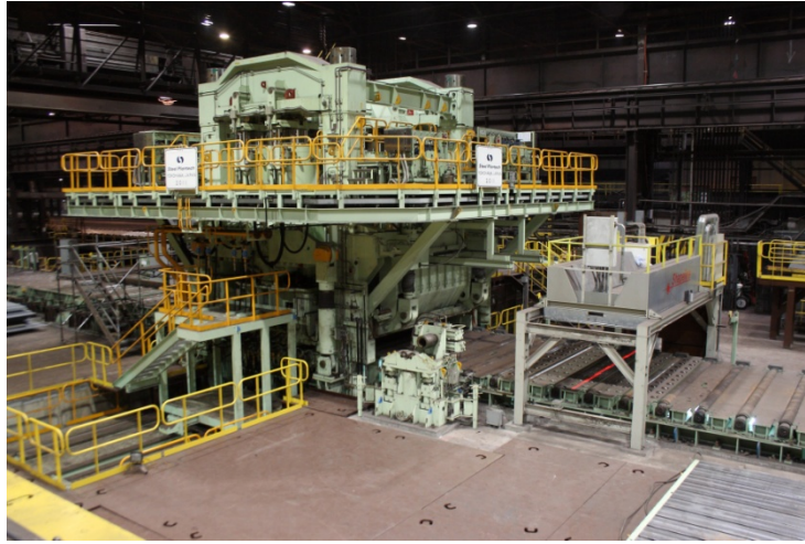
Figure 13. Heat treat leveler for AMBH (supplied by AMBH)
