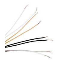
Straight In-Ear monitor cable formed from a durable TPE insulation material with robust Kevlar reinforced Litz cable for use by IEM manufacturers. Fitted with a gold-plated 3.5mm stereo audio connector; earphone connections are openended and tinned. A slider allows the cable to be held to the neck line.
