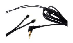
Straight In-Ear monitor cable formed from a durable TPE insulation material with robust Kevlar reinforced Litz conductors. Fitted with 2 pin gold-plated earphone connectors and a gold-plated 3.5mm stereo audio connector, Stainless-steel stiffeners are fitted to allow the cable to be formed around the ear. A slider allows the cable to be held to the neck line.
