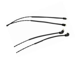
Figure-of-Eight Twisted In-Ear monitor cable formed from durable TPE insulation materials with robust Kevlar reinforced Tinsel conductors. Fitted with straight or angled 2 pin gold-plated earphone connectors and a gold-plated 3.5mm stereo audio connector, Stainless-steel stiffeners are fitted to allow the cable to be formed around the ear. Construction and special coating stop sweat migration and cable discolouration. A slider allows the cable to be held to the neck line.
