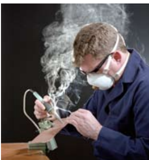
Figure 45 Soldering with and without Tyndall illumination
