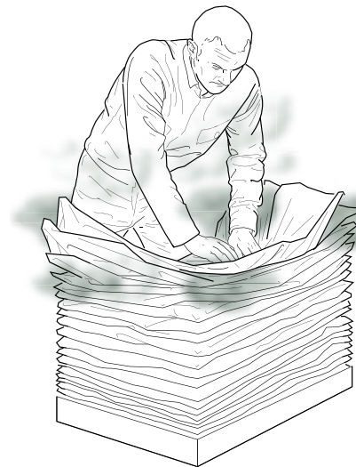
No LEV at sack crushing for disposal
