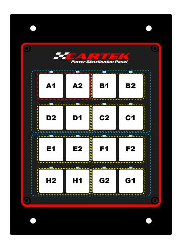
Each Channel on each Module can be set to any 1 of 8 selectable functions. However, when both Channels on a Module are set to the same function then extra functionality becomes available such as 'toggling' between Channels or synchronised flashing. Please refer to the Function descriptions later for more detailed information.
