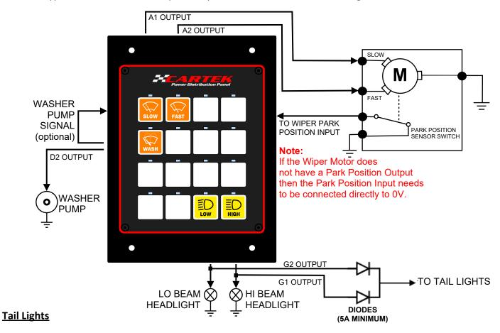
To make sure your Tail Lights operate when either Lo Beam or Hi Beam Headlights are used then please refer to the diagram above which utilises 2 Diodes.
