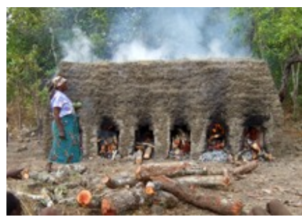
A brick kiln, which is burnt for 24 hours, uses three large trees to fire enough bricks for one small house
