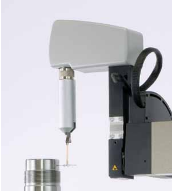
MDS3 with double-tipped probing system FT3 with collision protection
