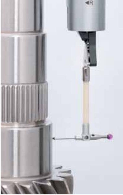
Measurement of roughness and form with double-tipped probing system and magnetic coupling
