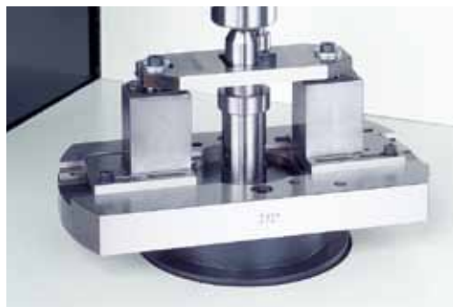
Workpiece-specific axial driver for cam shafts and crank shafts for angle indexing in axial bores
