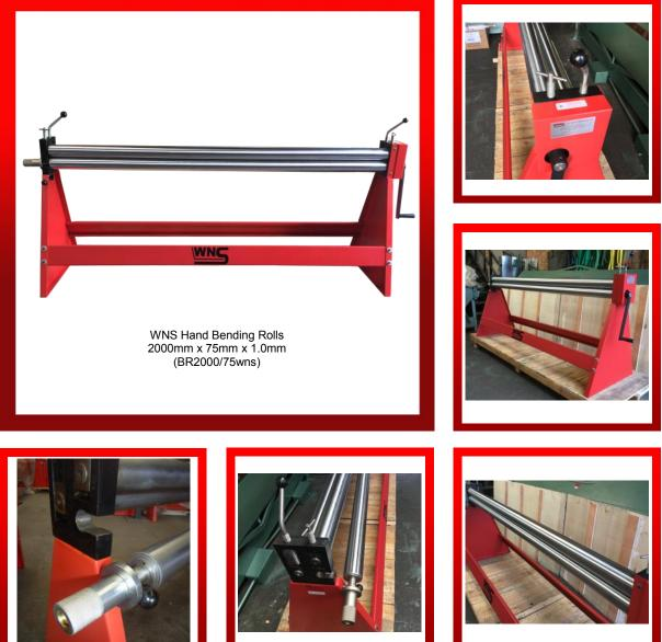
**WNS** INITIAL PINCH HAND BENDING ROLLS (BR2000/75wns) are principally used for rolling tubes/cylinders in sheet metal. The metal is 'pinched' between two rolls and curves as it comes into contact with the third (back) forming roll. The BR2000/75wns has a 2000mm Roll Length, 75mm Roll Diameter and can accommodate Mild Steel up to 1.0mm thick. The rolls are bottom slip, with an Edwards Style fabricated steel frame.
