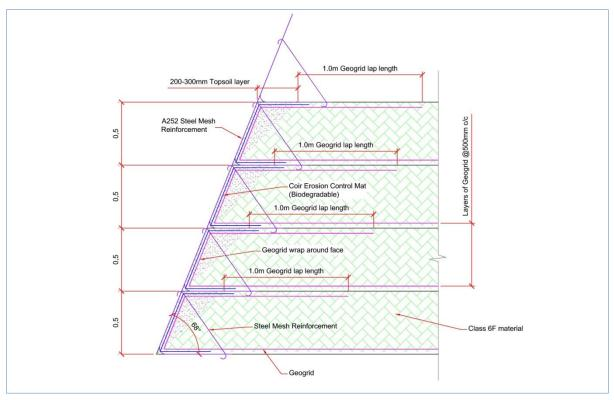
Figure 4 - Embankment construction details
