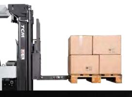
The SRO and SSO have the possibility for the addition of the telescopic forks, therefore becoming the SRT and SST. These trucks allow doubledeep handling to reduce aisle widths even further, or even loading and unloading transport from just one side. In some applications, this function can replace a small reach truck.
