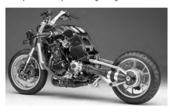
The steering head, upper plate and swingarm bracket were made stiffer, increasing torsional rigidity by 20 percent to reduce the influence
