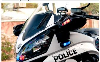
Windshield works in conjunction with air passages under the screen so that air flows more smoothly around the rider and helmet for a more comfortable ride.
