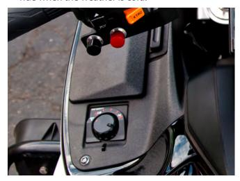
Stepless adjustment knob allows the heat level to be fine-tuned.
