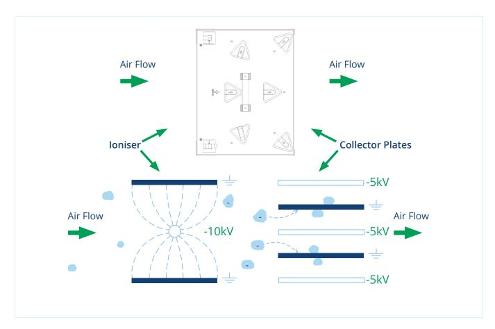
The above diagram shows, in a basic visual, how an electrostatic precipitator works. As air passes into the combined ioniser / collector cell, the particulates in the air stream are polarised to a negative potential. As they continue through the ioniser and between the collector cell plates, the polarised particulates are repelled away from the negatively charged plates and attracted to the earthed plates where they stick and so are filtered out of the air flow.
