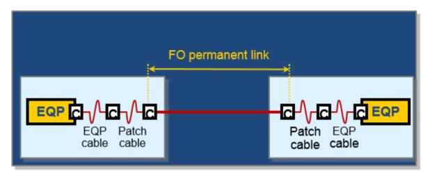
Sample of Permanent Link (EQP=equipment, C=connection)
