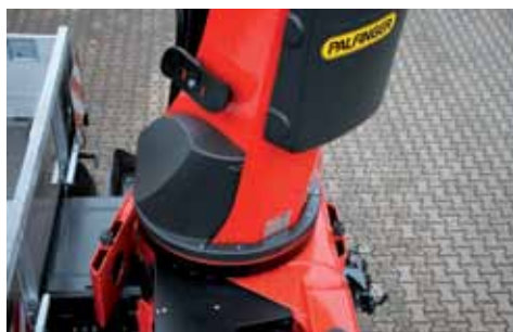
CONTINUOUS SLEWING SYSTEM UNRESTRICTED MOVEMENT
