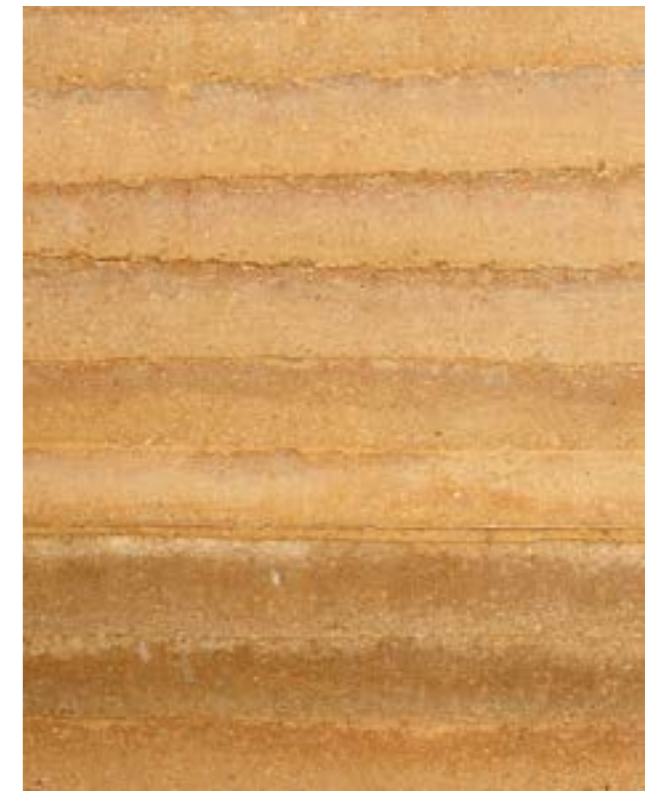
Custom Rammed Earth Sample (top right) Created by Clayworks
