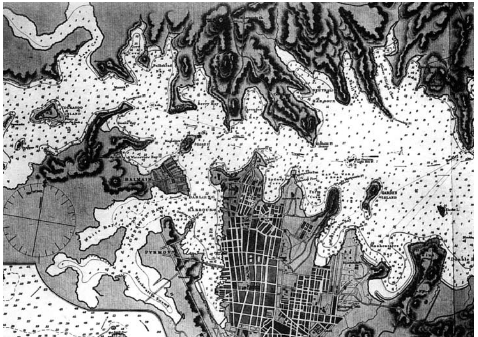
SURVEY OF PORT JACKSON 1857: The only existing survey had been carried out in 1822 and was badly out of date and inaccurate, so it was decided that a complete re-survey was necessary. A base of 2,780 feet was measured along the shore of Rose Bay and a triangulation scheme set up, with an observation spot on Garden Island, whose position was established as 33° 51' 58" S, 151° 15' 29" E. Extensive soundings were carried out from well outside the Heads to the upper reaches of the Harbour. Large-scale surveys of Cockatoo and Garden Islands were included so that accurate details of the docks and slips could be shown. The topographical survey of the surrounding land by Lieutenant Colonel Sir T L Mitchell was incorporated into the work, and the result is shown in the central section of the chart reproduced here, which was prepared by the Hydrographic Office in London, from the drawings and data sent by Denham.
