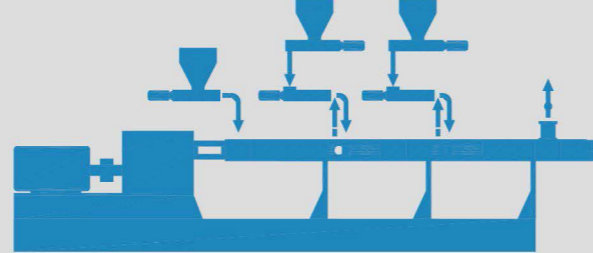
Filling and Reinforcing
