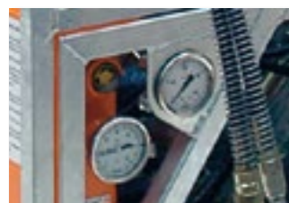
Oil temperature and pressure controls
