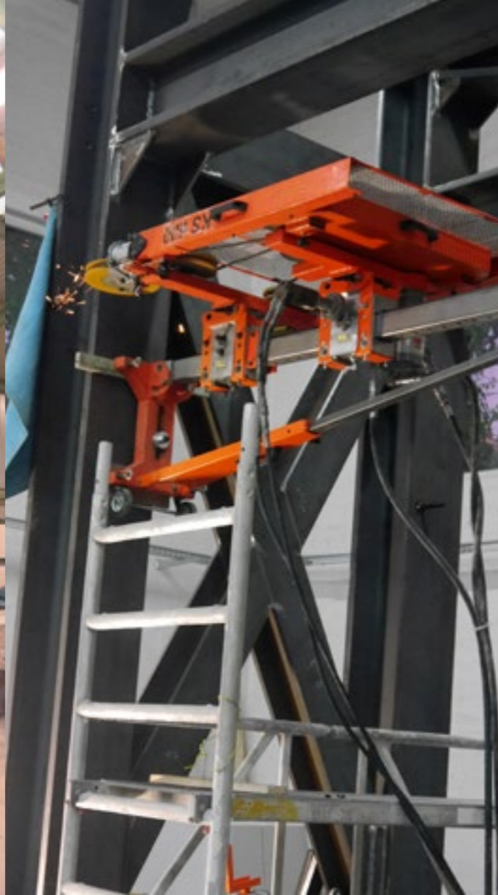
Wire sawing in heavy reinforced concrete as also cutting of STEEL PLATFORMS and STRONGBOX
