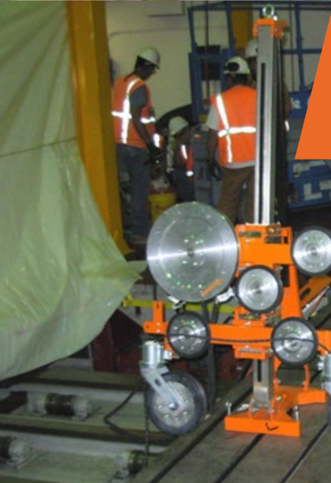
Wire sawing in heavy reinforced concrete as also cutting of STEEL PLATFORMS and STRONGBOX
