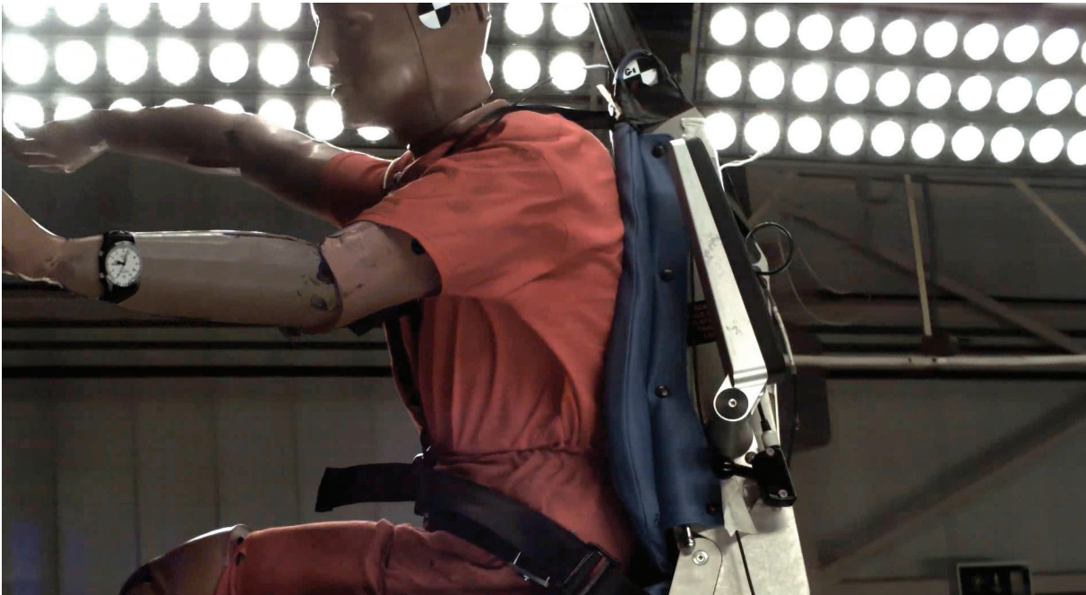
MFOS TEST - simulates a dynamic forward crash at over 18G, moving at 42ft per second
