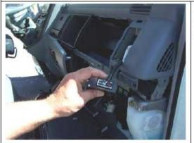
A Mitsubishi pulse converter is required for the control of the instrument cluster.
