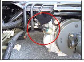
The original pulse generator is to be replaced by KITAS 2171-01000000.
