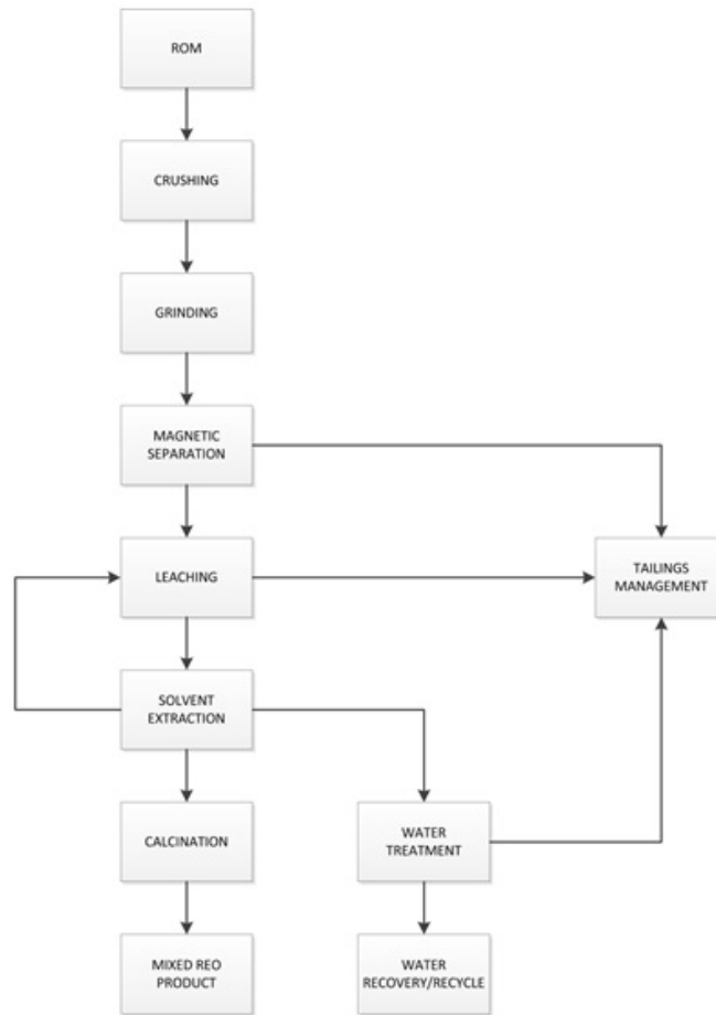
Figure 1: Processing Flowsheet for Norra Kärr
