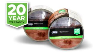
Trex Protect is a non-skid, self-adhesive deck flashing tape that is designed to protect the top of joists and bearers from moisture that can lead to timber rot and decay and the loosening of deck screws.
