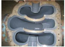
Casings coated with Belzona 1341 efficiency coating
