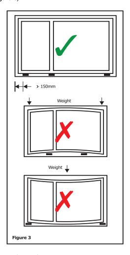
Support for the frame should prevent distortion and avoid damaging any protection or finish.
