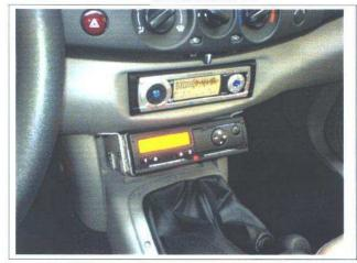
The DTCO is installed with the help of the installation console X39-140-000-011 underneath the radio compartment.
