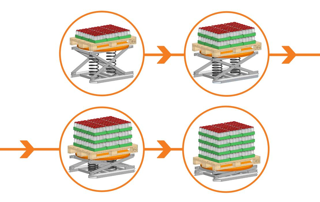
The Pallet Leveller automatically maintains a safe working height as load is applied
