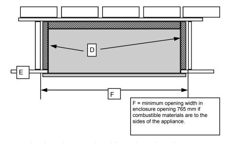
rear of the appliance location shall be protected with rigid non combustible insulating board or 50 mm thick rock wool or similar.
