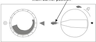
Main burner operational & thermostatically controlled
