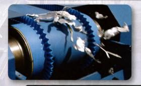
For applications that require separation of finer non-ferrous particles, Eccentric ECS units can be supplied. The Eccentric rotor differs in that the magnet system is of a smaller diameter and is located in an eccentric position to the outer rotor drum. The magnet system is positioned close to the surface, giving maximum repulsion where the conveyed materials discharge from the rotor.
