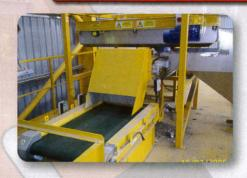
The Can Sorter is specifically designed for the separation of non-ferrous beverage cans from dry recyclable materials. The Can Sorter is a simplistic and cost effective solution providing optimum can recovery.
