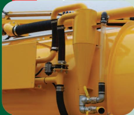
Hydro cyclone fitted to remove further debris particles from the recycled water.
