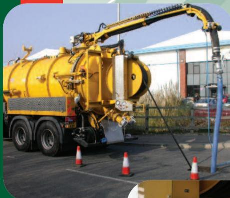
6" Pendant Operated Boom with Hydraulic Rotation extend and retract , Up and Down functions and Boom Valve Open and Close
