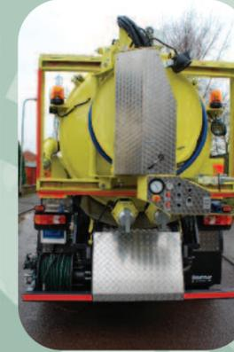
Main Reel Options available are 150 metres of 25mm on the Small Recycler and 150 metres of 32mm or 180 metres of 25mm on the Larger Recycler Machines. Also available is Traversing Reel option to shift the reel from side to side of the vehicle. Auxiliary Reel is 50 metres of 12mm fitted to the rear nearside of the vehicle.
