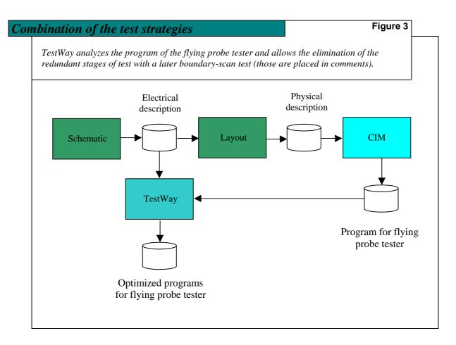
The TestWay testability analyzer generates two optimized programs for the flying probe tester: both have the same ability to detect a defect in combination with a boundary scan test. The difference between the two lies in the diagnostic resolution. The program version called Optimist considers that the JTAG tester will certainly be
