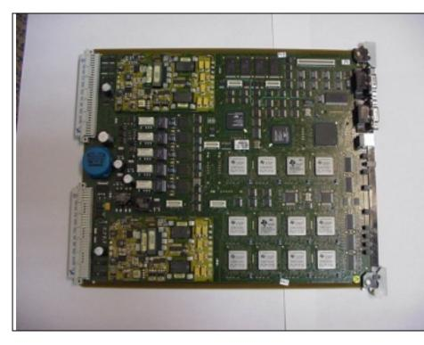
This board with 10 layers (board B of table II) includes many BGA and QFP with pin spacing of 50 mil and less. The combination of boundary scan test and flying probe test produces a minimal saving of 39% on the number of test steps.
