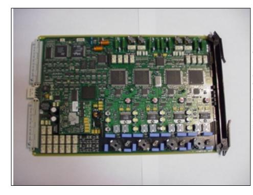
On this board with 8 layers (board A of table I), there are 1700 components, of which several QFP with the step of 20 mil. In spite of the small proportion of JTAG components (0,4%), the time saving carried out on the flying probe test exceeds 20% with the optimized program in its Pessimistic version.
