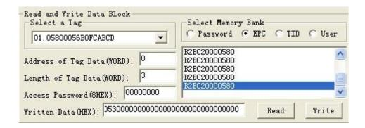
The fifth step, press <code>[read data]</code> button, reader began to read the label EPC number according to the first four steps setted conditions. The data displayed in the upper-right corner.
