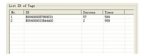
[Showing the identified ID] listed all the ID No. Has been identified. Remove the tag within the radio frequency area, can check the reading range.
