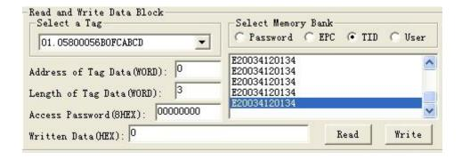
The fifth step, press <code>[read data]</code> button, reader began to read the labelTID number according to the first four steps setted conditions. The data displayed in the upper-right corner.
