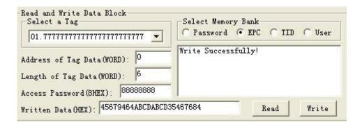
The fifth step, press [write data] button, reader began to write the label EPC data according to the first four steps setted conditions. The written data displayed in the upper-right corner.
