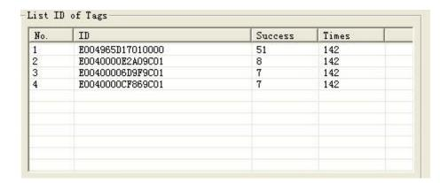
Remove the tag during the antenna radia frequency area can test the reading distance and range.
