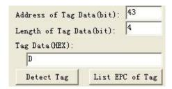
Fifthly, press <code>[identification tag]</code> button, reader began to read the label EPC number according to the first four steps setted conditions. Illustrate: see chart 5.1, radiation field have eight tags, If have to meet the conditions: data area initial address is 43, the data length is 4 (namely needs to compare 4), selected data of D, only card whose ID is <code>3005FB63AC1F3841EC885555 TID</code> area for <code>E2006004009AE045</code> meet the condition, and then showed as below:
