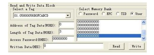
The fifth step, press [read data] button, reader began to read the label USER number according to the first four steps setted conditions. The data displayed in the upper-right corner.
