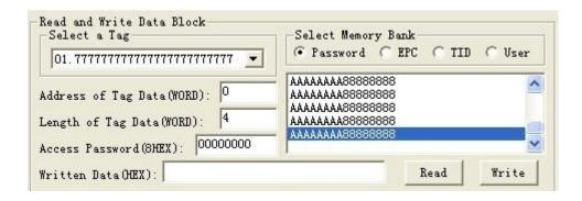
The fifth step, press [read data] button, reader began to read the label USER number according to the first four steps setted conditions. The data displayed in the upper-right corner. AAAAAAAA is kill password, 88888888 is access password.
