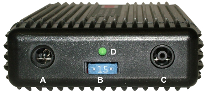
FIGURE D.1 A. INPUT JACK B. FUSE C. OUTPUT JACK D. LED (LIGHT EMITTING DIODE)
