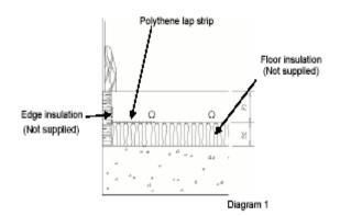
Note, some insulation board manufacturers recommend that you tape the joints to prevent screed ingress, which can form cold bridges.
