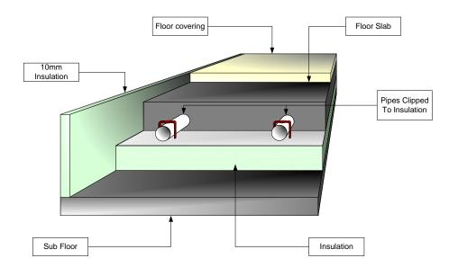
The Underfloor Heating system can be fitted in both concrete and timber suspended floors. See picture above. For other floor constructions please contact us and we will explain installation procedure, for example you can also do a floating floo
