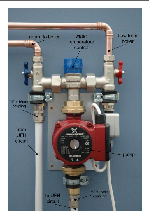
The Compact UFH System is designed for wall fixing and ideally should be mounted in a horizontal position with the electrical connection box uppermost. However, it can also be mounted vertical to pump up or down if desired.
