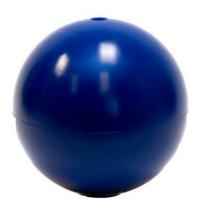
Spheres will pass through short bends, properly designed tees and fully-opening conduit type valves. They will pass through out-of-round pipe, will wear evenly, and can be wear-compensated by adjusting the diameter by inflating.
