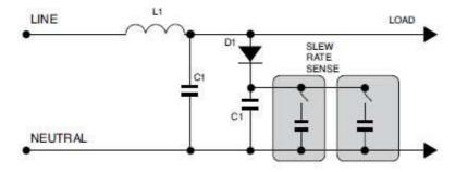
Simplified schematic of a series mode filter. There are no sacrificial components, so the filter does not wear down with use, and it repeatedly eliminates surges.
