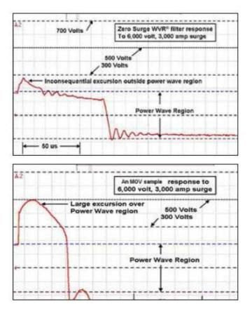
Two oscillographs of surge suppressors reacting to an incoming surge of 6000 volts and 3000 amps. Note the total time outside the power wave is high for the MOV.
