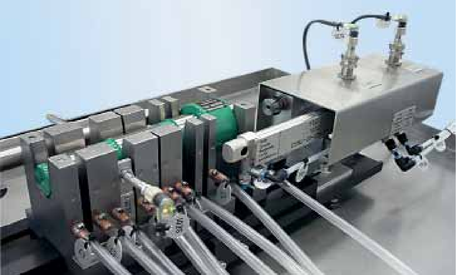
Application example with stand-mounted air snap gauges
