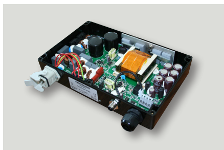
Power for roller conveyor. 150W with 500W peak power in IP54 enclosure.
