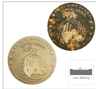
Laser Surface Cleaning
