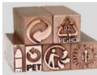
Deep Engraving on Copper Electrode
