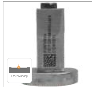
Traceability Mark for Automotive Part
