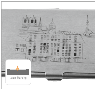
Laser Marking on Metal
