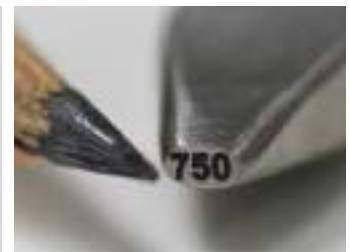
Micro Engraving on Hardened SS
