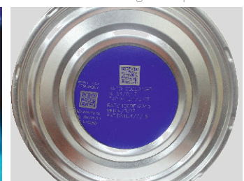
Laser Marking on Cap
