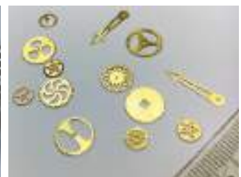
Micro Fine Cutting of Watch Part
