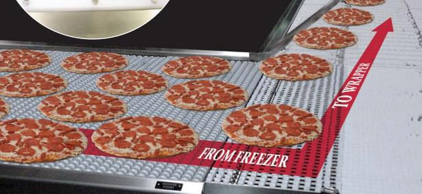
The low back pressure conveyor system gently accumulates and collates the frozen pizza products, without causing damage or shingling in a single rowing application.
